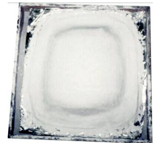
Figure 11: The completion of the fiberglass and hydrocal application.
