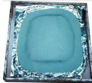
Figure 8: The specimen and the flange, layered with the rolled clay.
